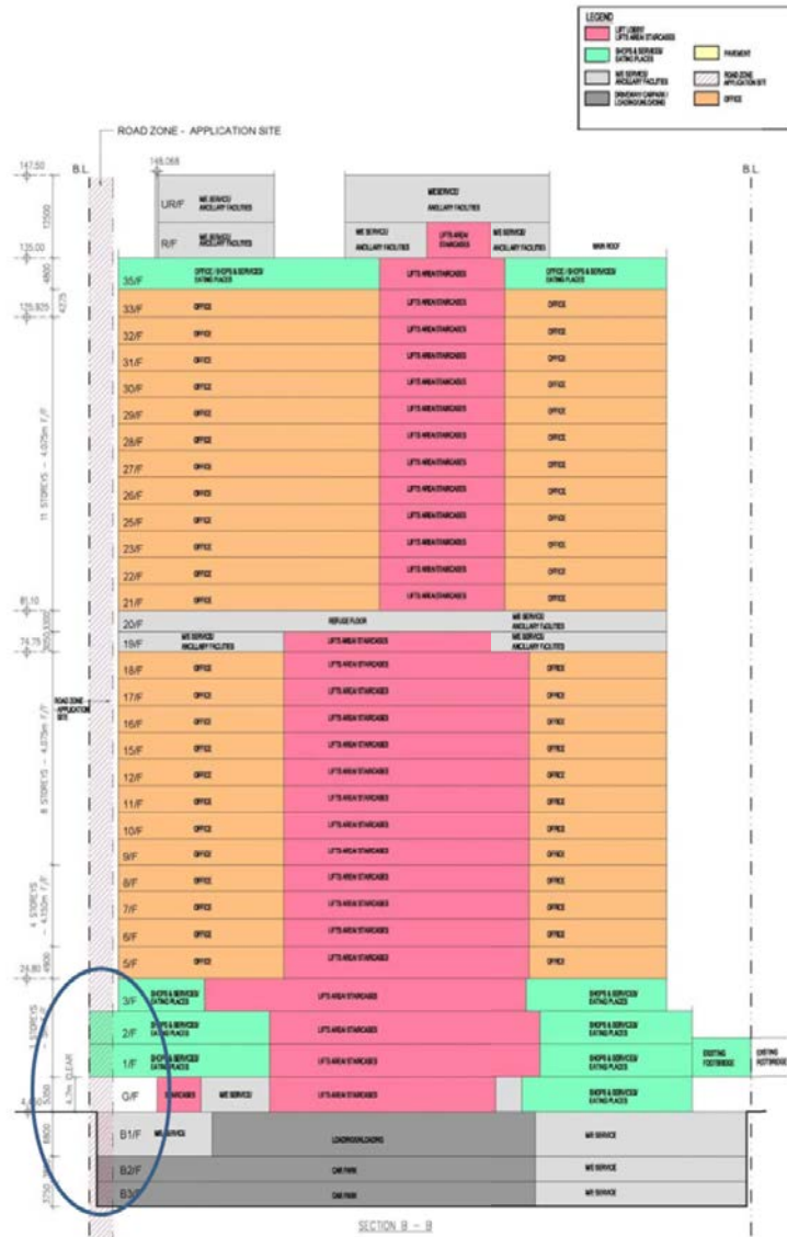
Figure 8: Section B – B of the Proposed Scheme, showing on the left, the building extending into the Application Site at all three basement levels and the over-hang at the 1/F and 2/F portions of the tower. The levels above the 3 rd floor are set back from the “Road” zone. The G/F is also set back, complies with the limit of the “Road” zone, and the clear headroom will permit vehicle movements.
