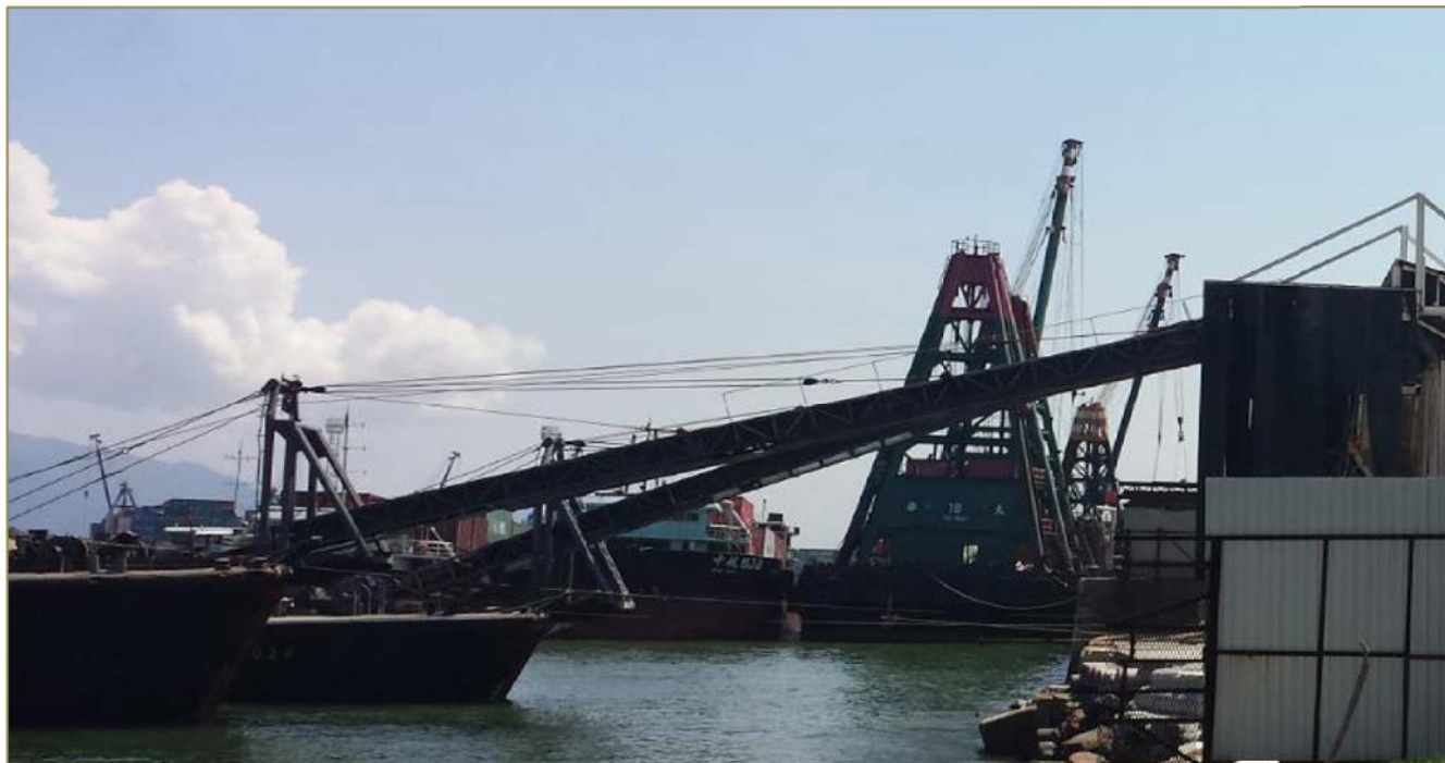
Figure 4.1 A typical Pelican Barge Unloading Operation
