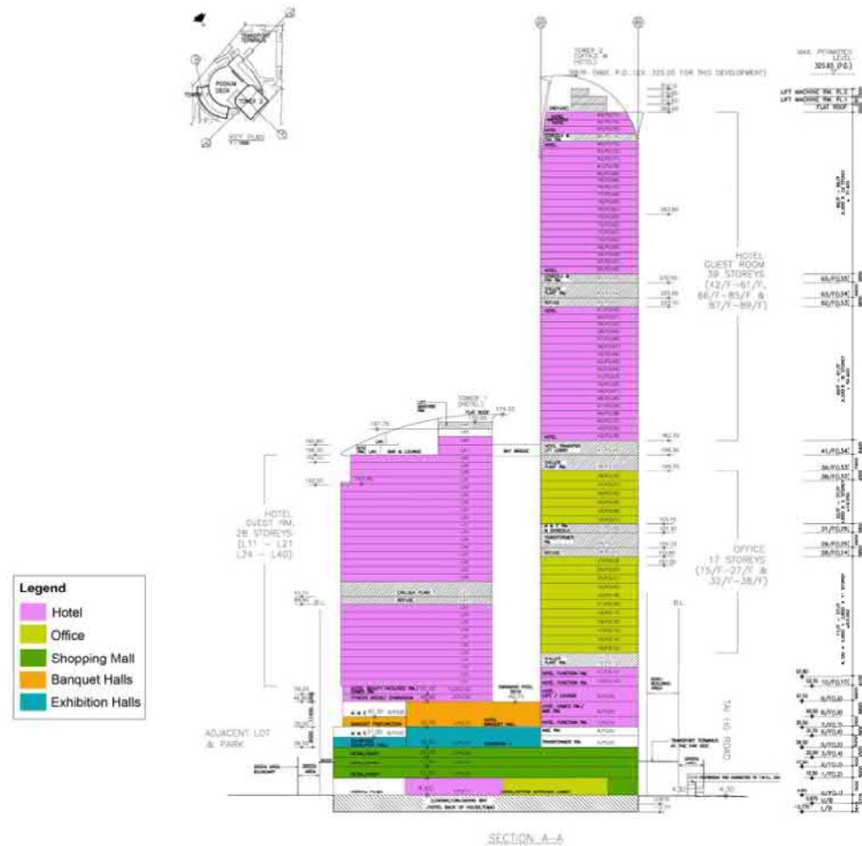
Figure 2.2 Diagrammatic Section of the Existing Floor Uses at Nina Tower
