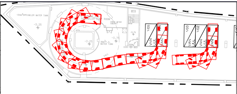
Swept Path of Small-sized LGV Exiting L/UL Bay and on Up-Ramp
