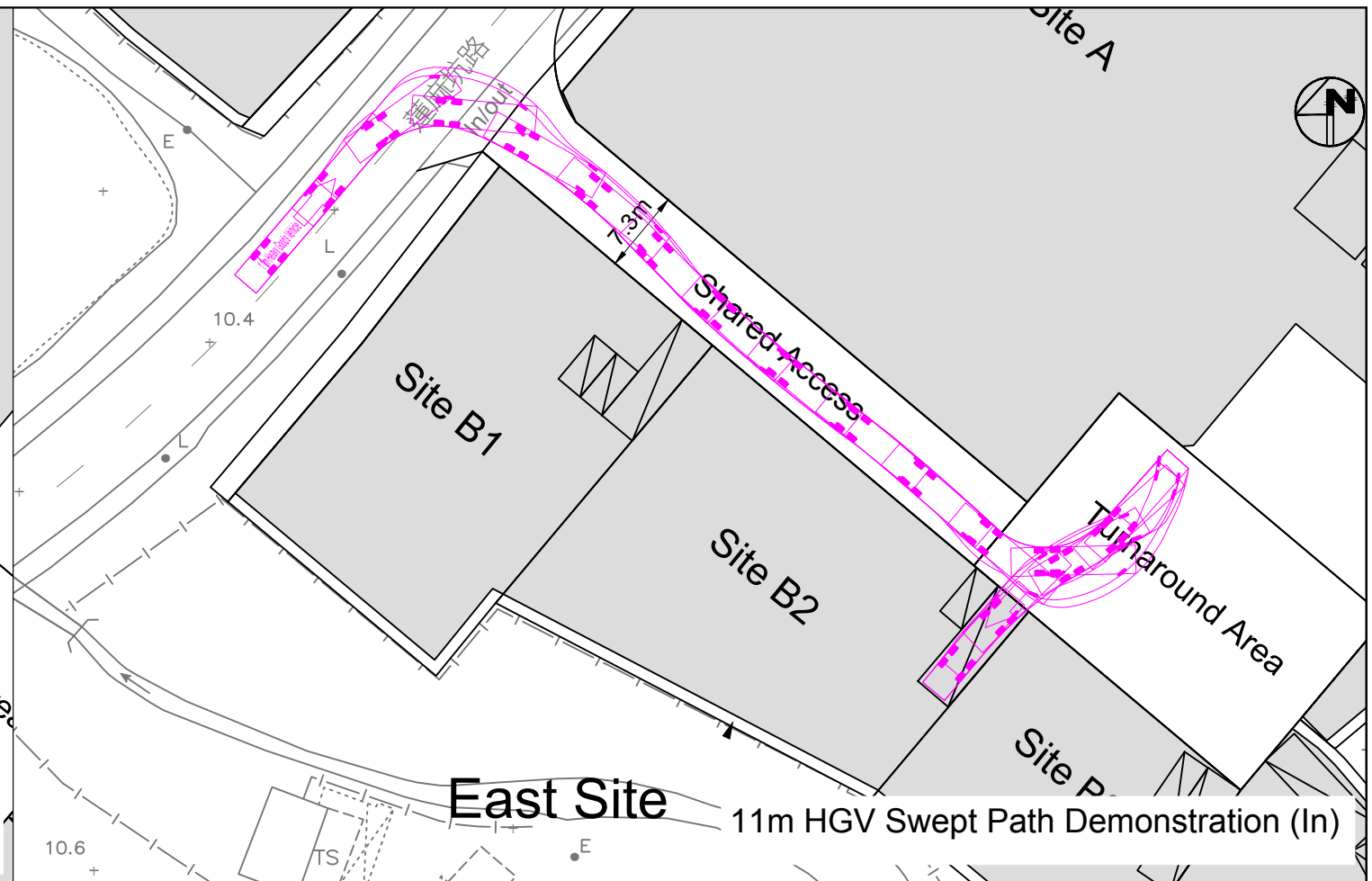
11m HGV Swept Path Demonstration (In-Step 1)
