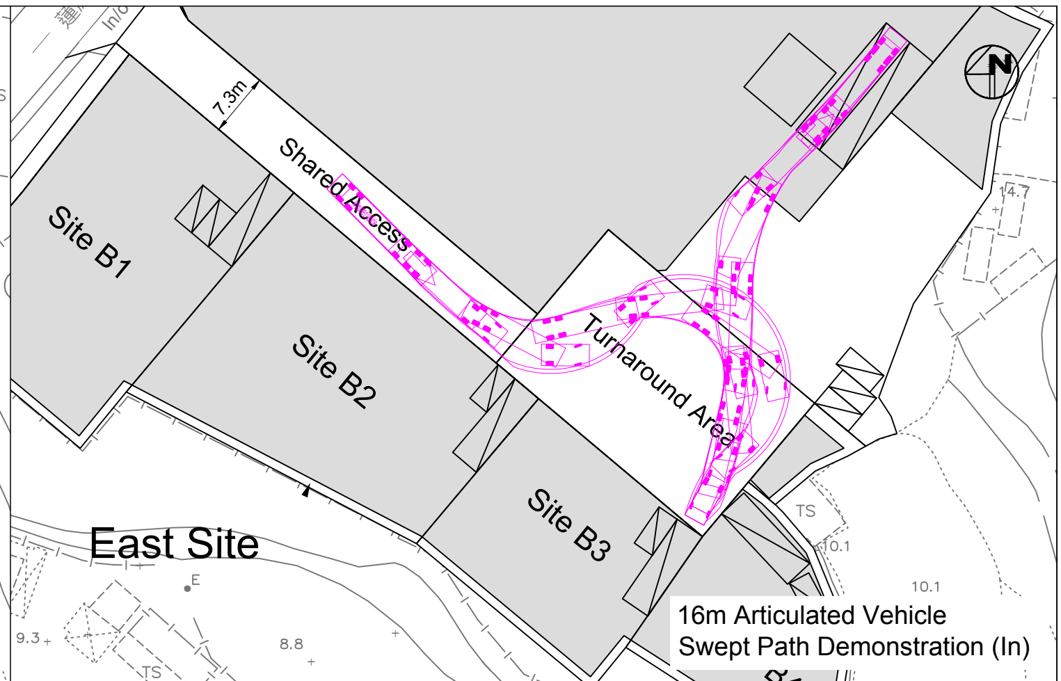
16m Articulated Vehicle Swept Path Demonstration (In)
