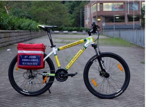
First Aid bicycles are custom made with a longer bicycle frame in order to facilitate easy usage when first aid boxes are attached to both sides of the bicycles. Since they are custom made, they would have to be securely stored during non-operational hours. Also due to their field patrol nature, they would have to be stored separately (in <u>Unit 2</u>) for hygiene reasons to avoid contamination of the treatment unit (<u>Unit 1</u>).
