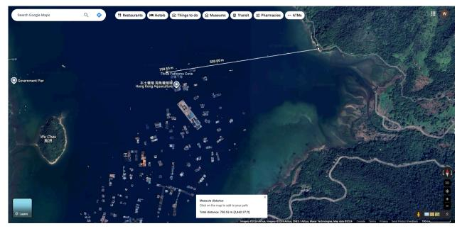
However, there are also fish farms in the middle of the zone which may not be able to acquire adequate and stable supply of electricity. In consideration of these fish farms, we measured that the possible cabling plan towards the northwest of the zone is 1000m (rounded off) in length, with 5% added buffer it will be 1050m.
