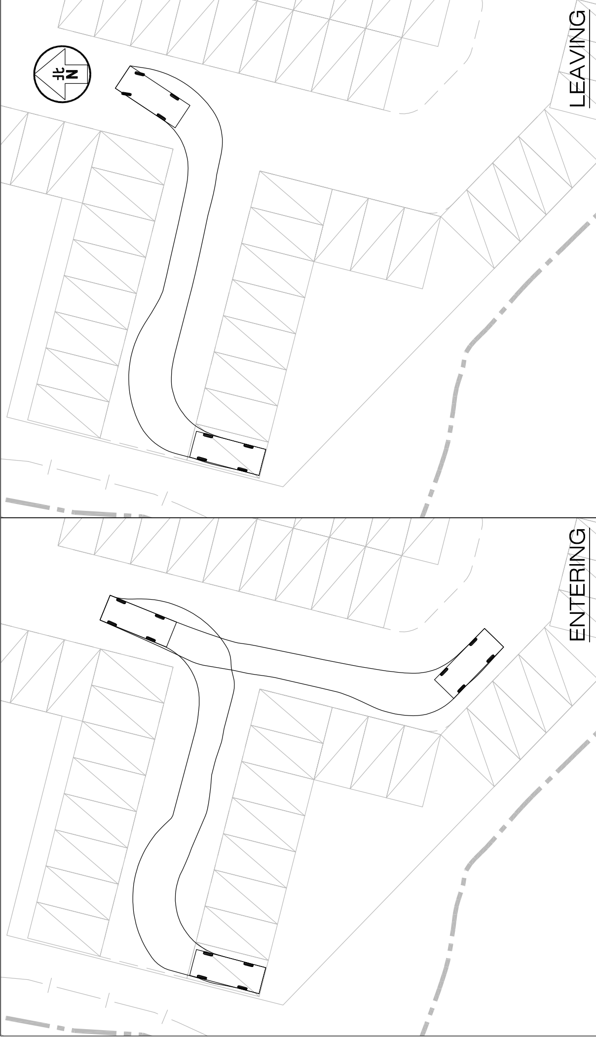
SWEPT PATH OF PRIVATE CAR ENTERING AND LEAVING THE PROPOSED TEMPORARY CAR PARK
