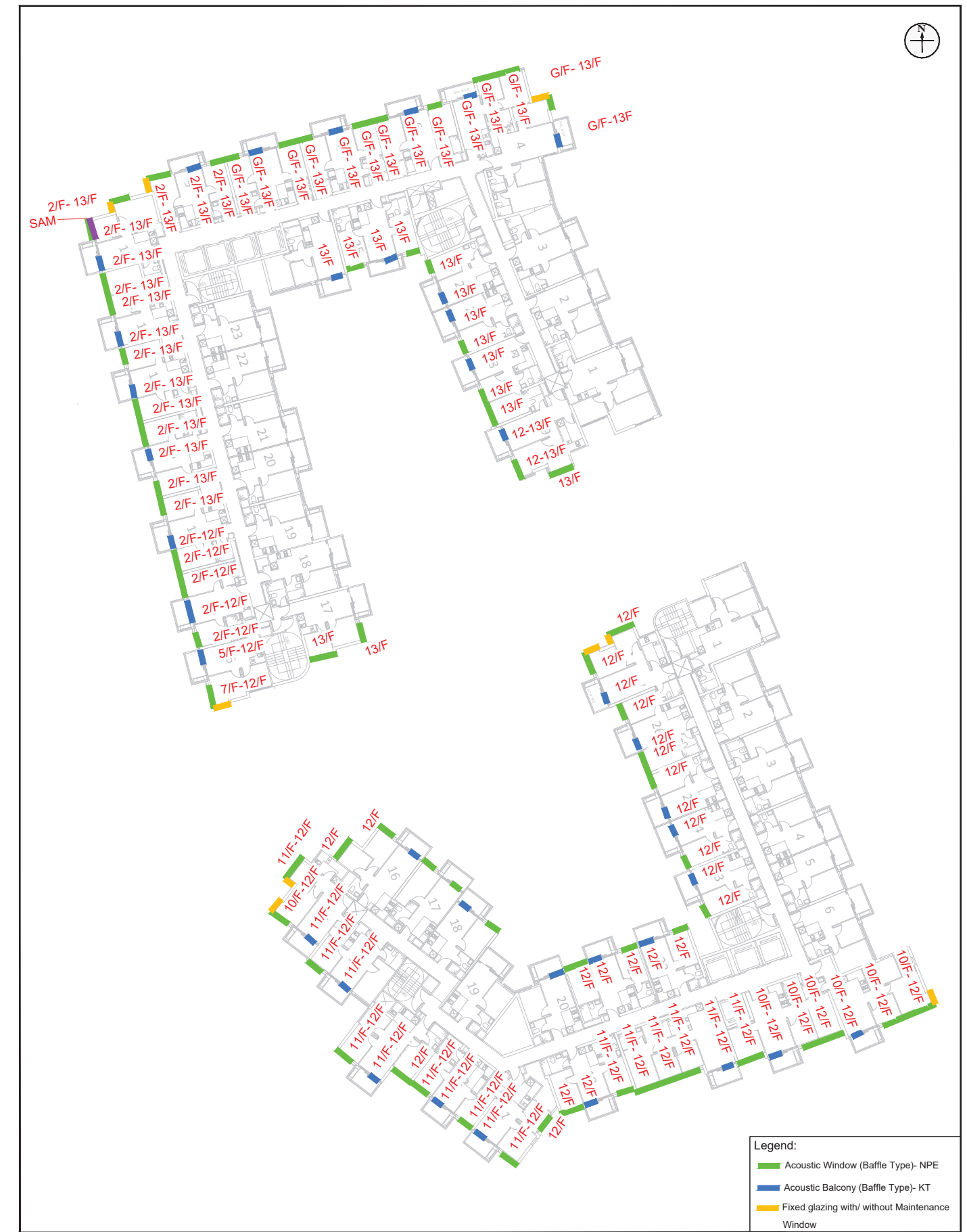
Figure: 2.2 Title: Location of Proposed Noise Mitigation Measures (T1 & T2) Project: Section 16 Planning Application For Submission of Layout Plan For Permitted 'Flat' and 'Social Welfare Facility' use at Tsuen Wan Inland Lot 5 and Lot No. 429 In D.D. 399, Ting Kau, Tsuen Wan
