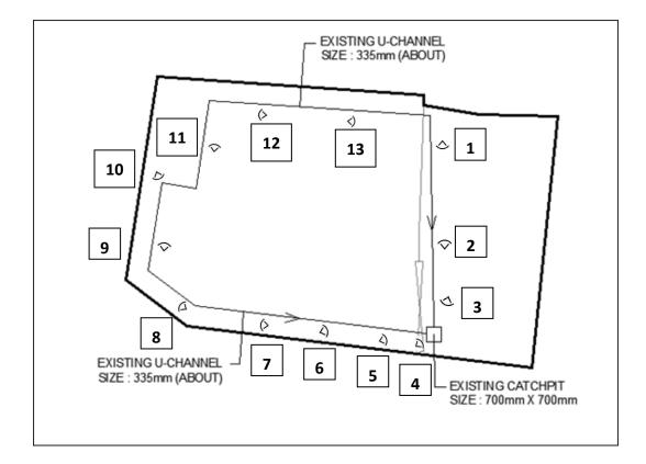
i) The as-built drainage plan showing the existing drainage facilities at the Site:
