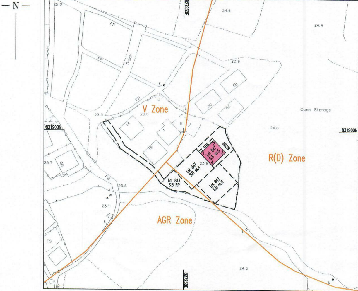
Figure 5- Plan Showing the current Zoning and Location of the Septic Tank and Soakaway System
