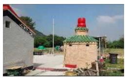
Photo 4: Burner at the temple is enclosed type with solid walls on 3 sides (size around ~2m wide and ~2m high).
