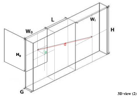
(for case that inlet (outer) opening height is different from outlet (inner) opening height, applicable to window with sliding panel behind (baffle type acoustic Window) for the proposed development)
