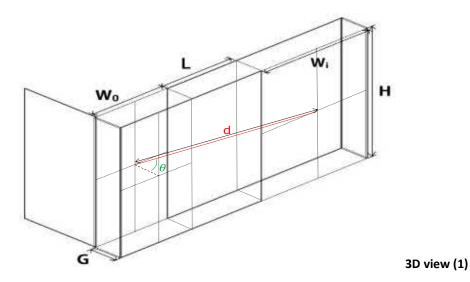
(for case that inlet (outer) and outlet (inner) opening heights are the same, applicable to living room door with sliding panel behind (baffle type acoustic Window) for the proposed development)
