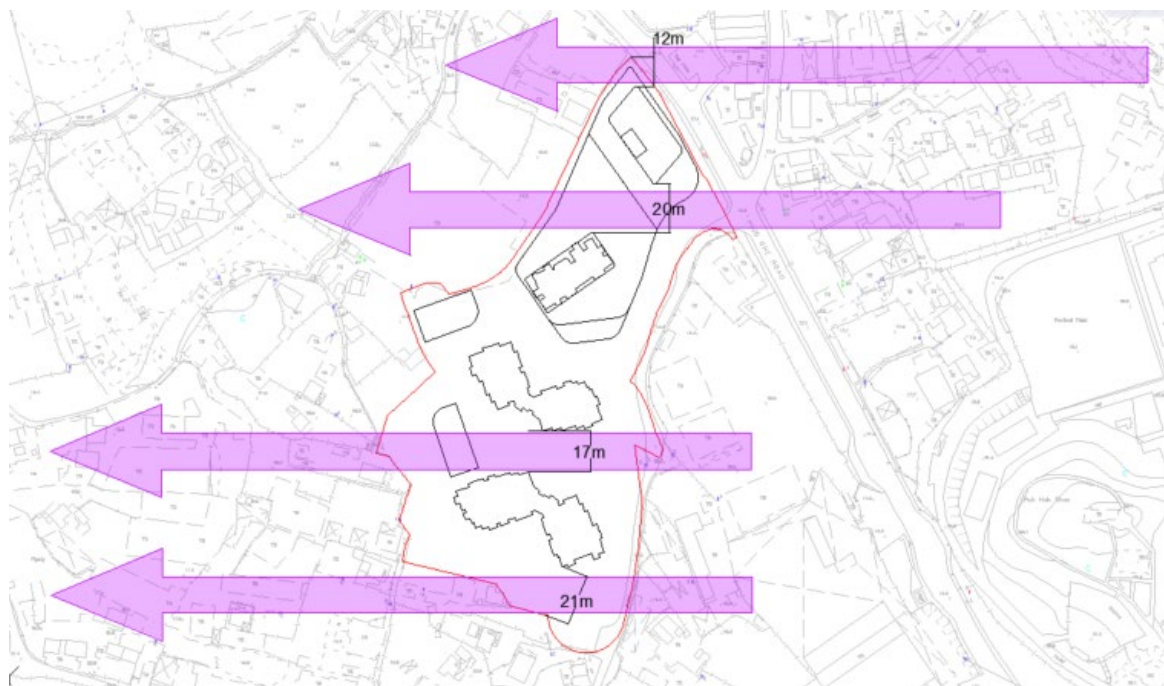
Figure 5-3 Zoom in plan for the E wind flow pattern
